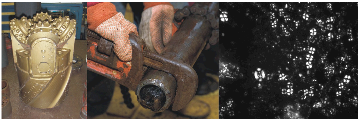
RCB drilling head (left), core catcher with chert piece (middle), Cretaceous coccoliths (right, magnification: 63x, crossed polarized light).
